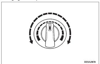
Select the desired temperature level by turning the temperature control dial either clockwise or counterclockwise. Turning the temperature control dial clockwise makes the air warmer.
